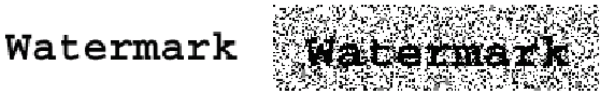
Figure 3.1: A black and white pattern watermark before and after additive noise
